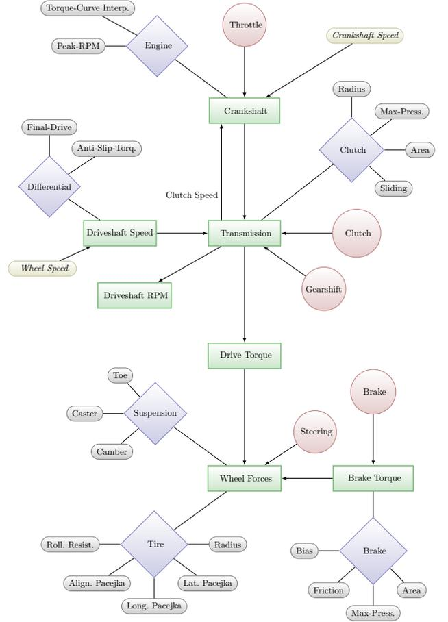
Fig. 1. Overview of VDrift's car model
