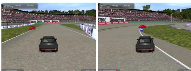
Fig. 6. Application of the open loop controls to the leading red car in VDrift leads to violation of track constraints, making the need to include feedback information obvious.
